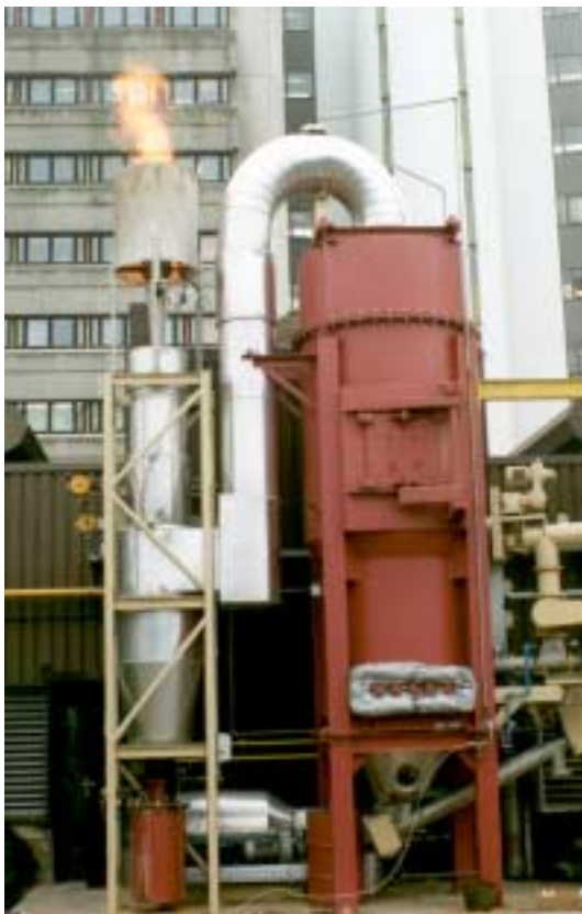
Figure 14 Pictures of the externally fired gas turbine plant: the gasifier flaring the gas (left) and the gas turbine with the external firing arrangements (right)
