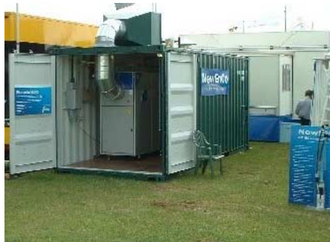
Fig. 6 NewEnCo's biogas fired microturbine package[www.turbec.com]
